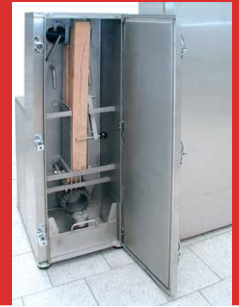
FVK friction smoke generator – VERTICAL
